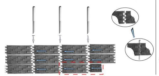
5. Fold the panels up to meet and stand the whole structure up with half panel at the bottom
